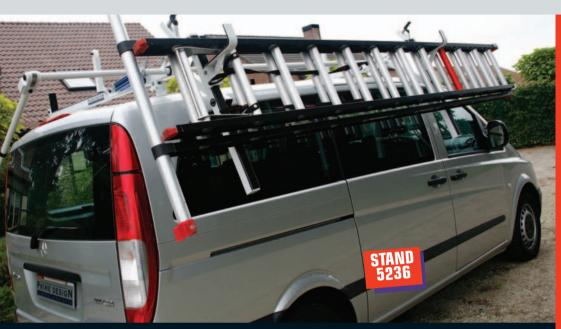
**Prime Design Europe** is looking to improve its presence in the UK market with a range of lightweight roof storage solutions. The latest product in the range is Ladderlift ErgoRack, which allows the operator to stay on the ground while loading and unloading ladders. Also on the stand will be the company's aluminium roof racks and bars.
